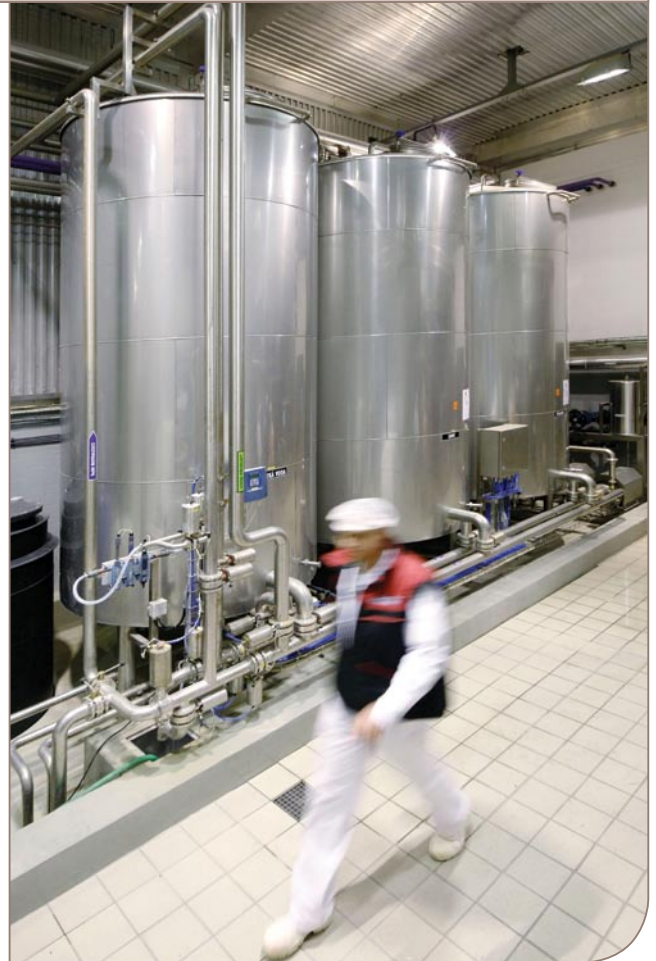
Modularised skid mounted plug-in unit for automated Cleaning-in-Place.
