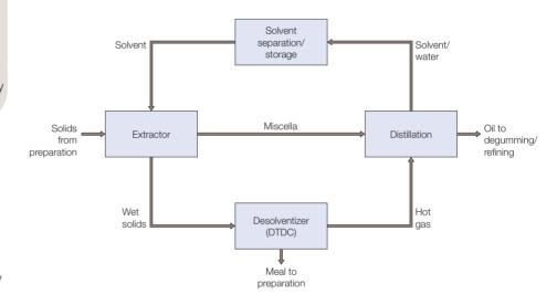
The solids are typically processed in a unit called the desolventizer (DTDC), whose main function is to flash the volatile solvent from the solid phase by use of direct steam injection. The vapour leaving the DTDC must be cleansed and condensed.
