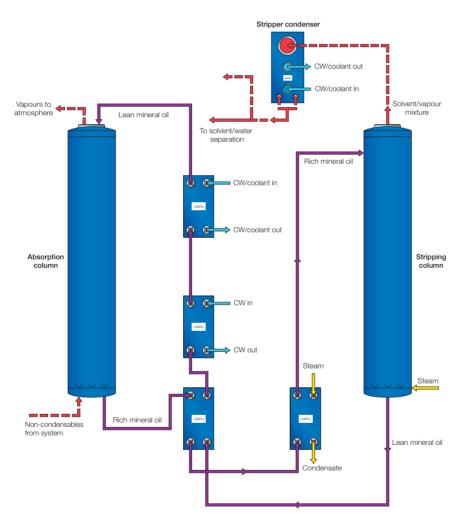
Example flow diagram - Vapour scrubbing
