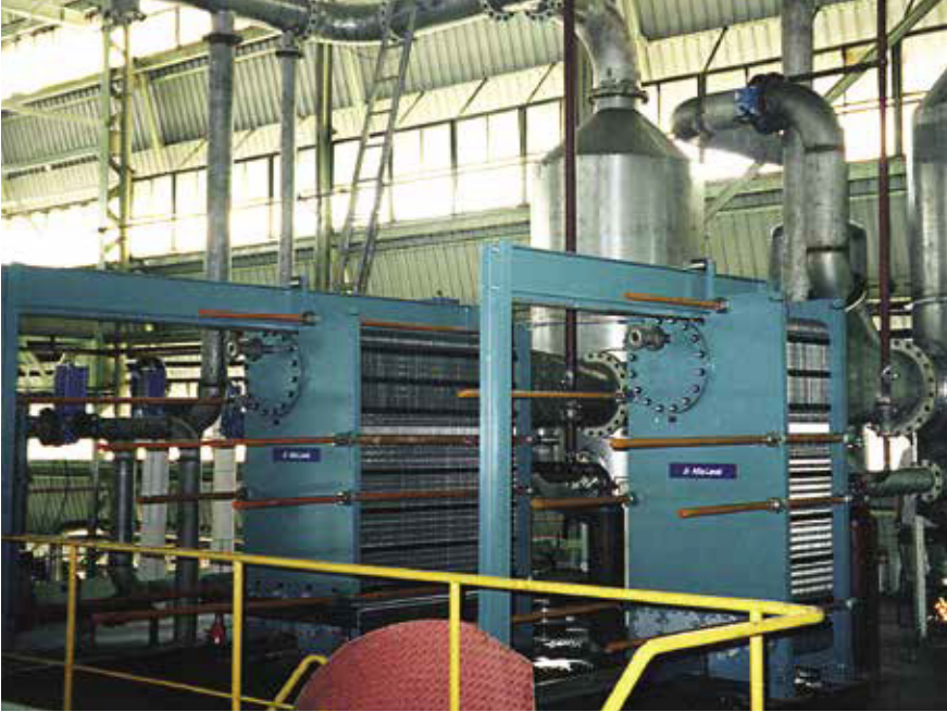
AlfaVaps used in a two-effect TVR system in a sugar refinery in Malaysia. An existing parallel falling film shell-and-tube system can only deliver fine syrup to a concentration of 71 Brix. The AlfaVap system concentrates all the way to 75 Brix without recirculation, achieving a very short processing time. This results in a better product quality, and provides simpler and faster start-up and shut-down procedures.
