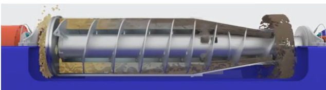
Figure 2. Shallow cone configuration
