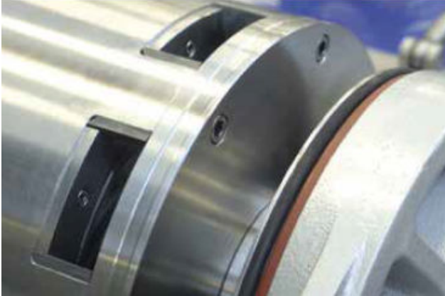
Figure 3. Solids discharge, free from blocking
