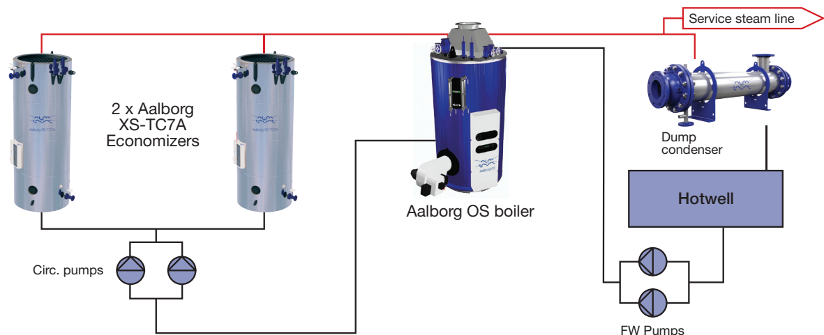
EMMA MÆRSK equipped with the Alfa Laval Aalborg XS-TC7A waste heat recovery economizer.
