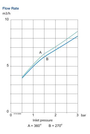
For Clip-on models, the flow rate is increased by approx. 0.5  $\ensuremath{\text{m}^3/\text{h}}.$
