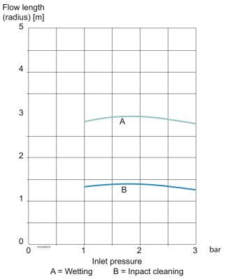
**Note**: The inlet pressure has been taken immediately before the inlet to the machine. In order to achieve the performance indicated on the curves, the pressure drop in the supply lines between pump and machine must be taken in consideration and the water temperature during testing was approx. 20 °C.
