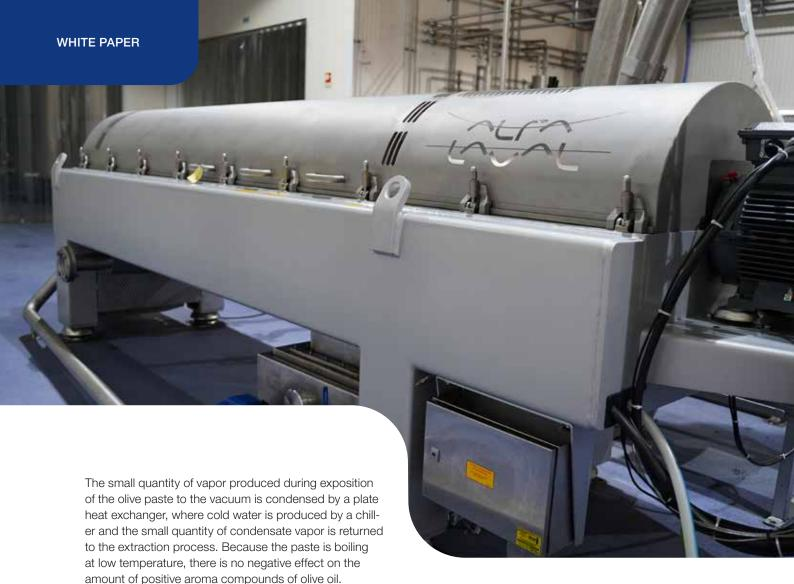
This step of "free oil" release could be obtained entirely by the Olive Oil Booster, or by using the booster in combination with traditional malaxing.
