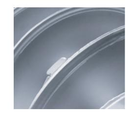
Figure 6. Flame sprayed tungsten carbide wear protection on conveyor flights
