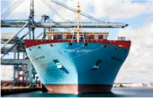
The Triple-E's wide, U-shaped hull and more bulbous bow mean it can carry even more containers.
