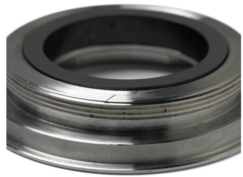
Poor quality of non-genuine shaft seal. A cheap purchase, but expensive to replace.
