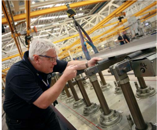
An employee at Airbus, Broughton's wing assembly plant inspects an aluminium stringer.
