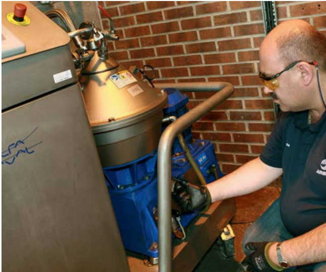
An Alfa Laval AlfaPure Z3 used for cleaning coolant in the stringer manufacturing shop at Airbus, Broughton.
