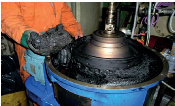
Figure 13. A separator subjected to instable fuel.
