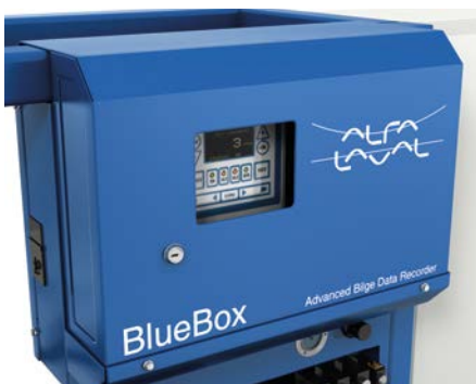
PureBilge BlueBox with the EPC 60 Bilge operator panel.
