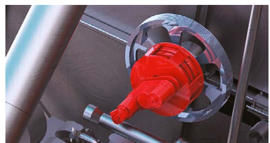
Vspeed variable fan drive minimizes power consumption.
